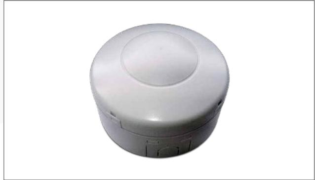
The MV-01- IP Microwave detector is a standalone version of the MV-01 and is used for applications where a sealed detector is required. It is supplied within a circular housing which is suitable for direct mounting to a solid surface and has BESA box fixings for conduit applications.
